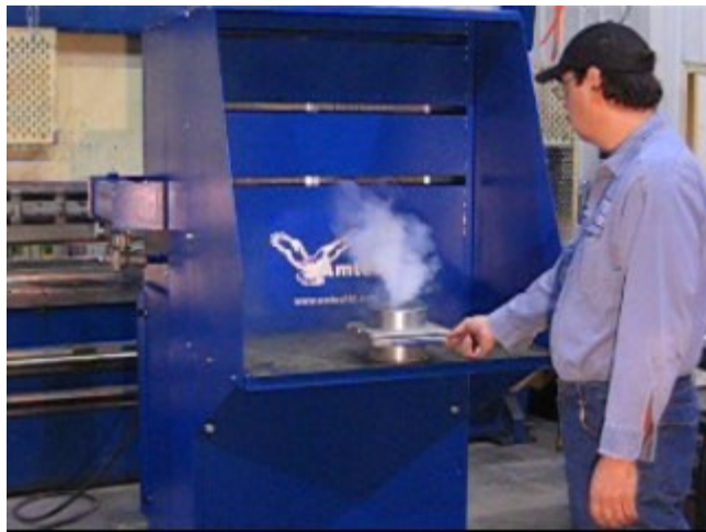
Removes Contaminates from the Breathing Area of the Operator.
