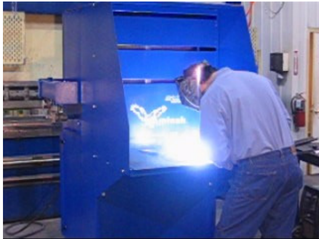
Captures Welding, Grinding and Polishing Fumes and Smoke.
