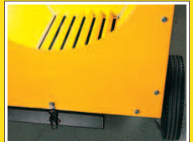
Dust baffle eliminates back suction.
