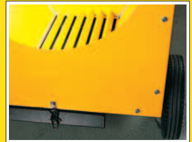
Dust baffle eliminates back suction.
